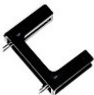
Two photogate cables are supplied. The cable with the black U-shaped piece shown to the left (called an interrupter) is convenient for triggering on smaller drops or vibrating strings. For the passage of larger objects, use the photogate cable that has a separate emitter and detector. (The emitter has the blue case.) Both photogate cables have 3 wires: red, black, and green. Connect them to the breadboard at the locations given in the table.
