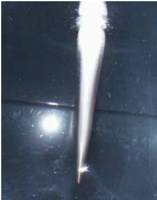
In this photo the BB has entered the water from above, and is the blurred copper colored streak near the bottom of the image. The cavity left behind is clearly visible, but is quite blurred.
