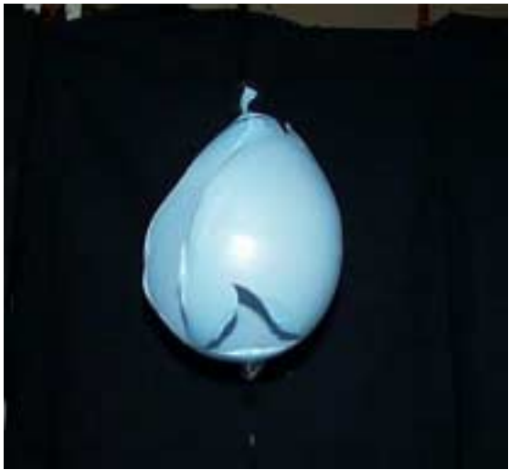
The BB has just passed through the balloon, and is visible at the bottom of the frame, having been shot from above. The balloon has ripped up one side completely, and a partial rip is visible in the center.
