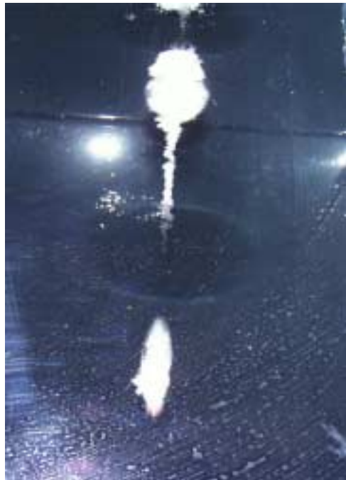
This image was taken at a later point in the water entry, and the cavity left has separated in the middle. Less blurring in this image is likely the result of slower speeds.
